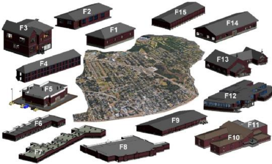
Figure 4. Schematic representation of using minimum building archetypes portfolio to model a community.
